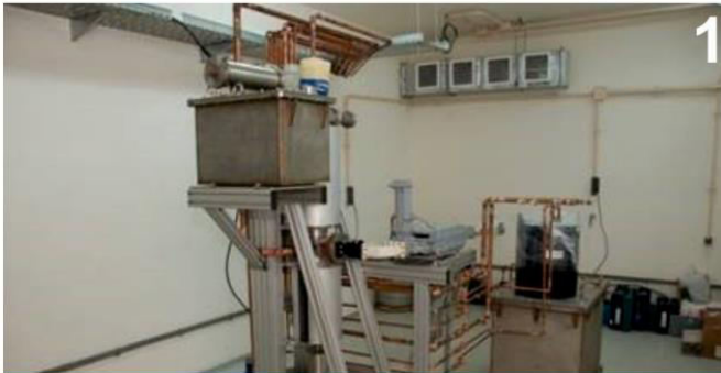
Linear electron accelerator УЛЭР-10-10С. Particle energy is 10 MeV, beam current is 1 mA, output power is 10kW
